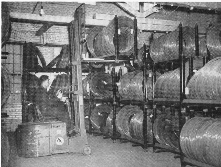
Above is a photo of the Lewis-Shepard lift truck now in use in the Wire Storage Department of the Waterville Division. This lift truck enables the stacking of special wire pallets three tiers high, or approximately nine feet. Floor space is thereby more effectively utilized.
